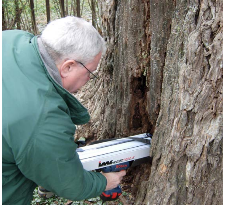
Resistograph readings provide measurable data to help make informed decisions about a tree or structure.
